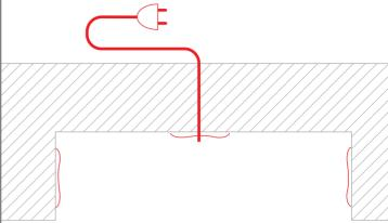
${\bf 3.}$  Connect power to the LED strip and mount the extrusion (A) in the mounting groove.
